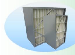
**EARB-DP** is the 1<sup>st</sup> generation of Rigid Box filter created, and the only rigid box type that uses Synthetic media. Using a similar concept as pleated filters, the media is designed in deep pleat with a metal casing, to increase its rigidity. EARB-DP is the best economical choice among rigid box filters, commonly used for Commercial Building applications.
