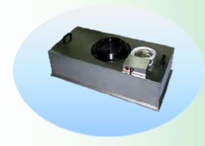
**EAPA-FFU** is commonly used in cleanroom applications, especially for Class 100 and below. It is used extensively in laminar hoods and research centres. It comes with a fan motor in the unit itself, together with a Mini-Pleat HEPA at the bottom of the casing.
