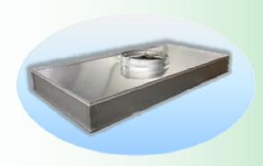
**EAPA-TM** is vastly used in cleanroom and hospital applications. Differ from EAPA-FFU, EAPA-TM does not come with a fan motor in it. As such, the casing profile is much lower. Similarly, EAPA-TM comes with a Mini-Pleat HEPA at the bottom of the casing.
