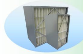
**EARB-DP** is the 1<sup>st</sup> generation of Rigid Box filter created, and the only rigid box type that uses Synthetic media. Using a similar concept as pleated filters, the media is designed in deep pleat with a metal casing, to increase its rigidity. EARB-DP is the best economical choice in the rigid box filter range, very commonly used for Commercial Building applications.
