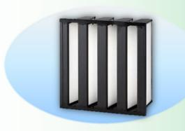
**EARB-V** is designed using the latest state-of-the-art technology. Built in a V-shaped construction, it allows EARB-V to increase media area tremendously for maximum usage, while sustaining a low initial pressure drop. The unique plastic frame makes the filter light in weight and easy for handling during installation.
